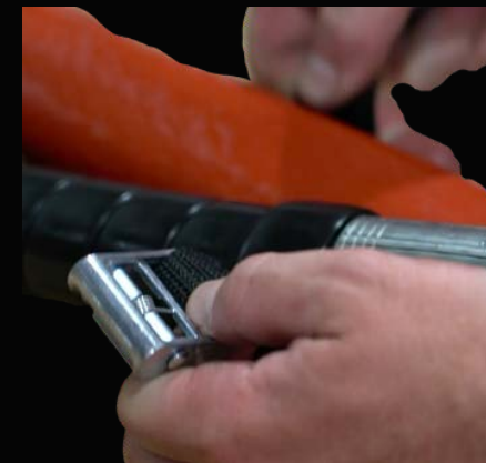
2. BRING BUNDLING STRAP UP FROM UNDERNEATH/BEHIND THE HOSES
