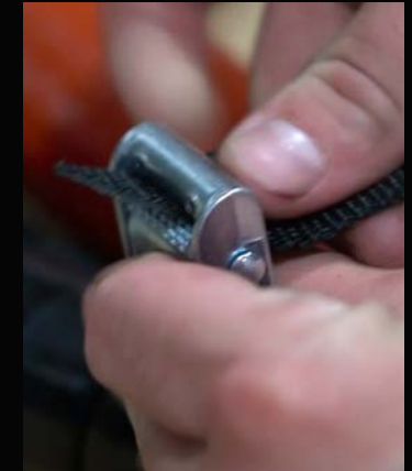
3. THREAD THROUGH THE HEAD AND PULL TIGHT. There should be no room for a finger to get underneath the strap.
